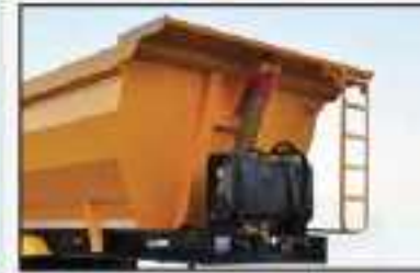
Hydraulic Tank, Cylinder, Ladder
