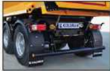
The tailgate auto-locking system. Rear bumper, steel bar foldable type.
